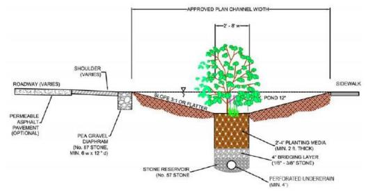
the base of the media trench if soil infiltration is inadequate to drain the swale. The underdrain should include a capped cleanout pipe to allow for flushing as necessary.
